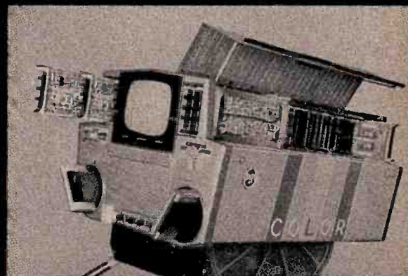
Transistorized modules afford easy servicing, are more reliable, and provide highest performance.
